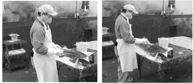
A laminator wetting out the mat with resin, then rolling out air pockets with a special roller.
