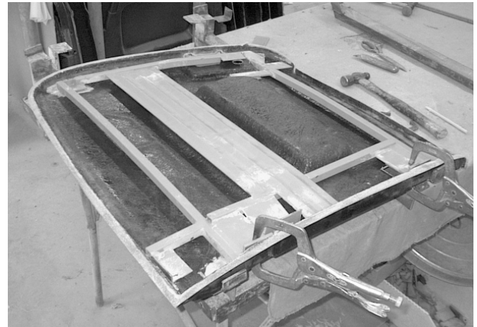
Steel installation inside a '34 roadster door
