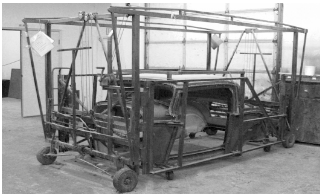
1932 3-Window mold inside the lifting and rotating mechanism
