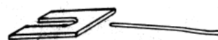
Use a U shaped shim for fitting. Attach a wire "tail" for easy removal. Replace with washers when done
