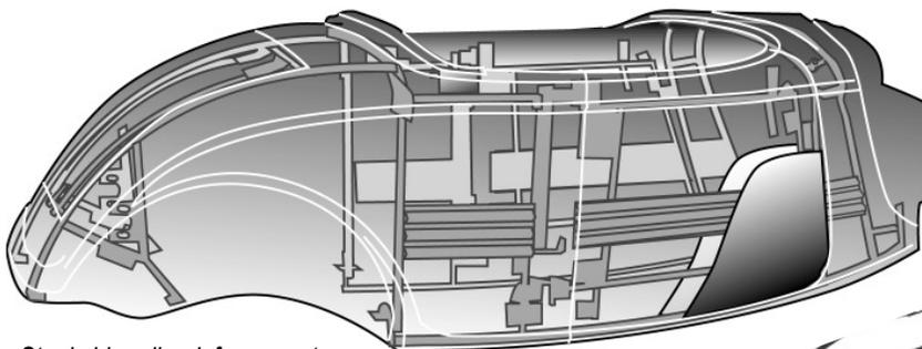
Steel side rail reinforcement from cowl to rear of cockpit
