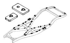
1932-47 Pickups used a heavy wood body to frame spacer block. The proper shape and spacing are important for proper body to fender and hood alignment.
